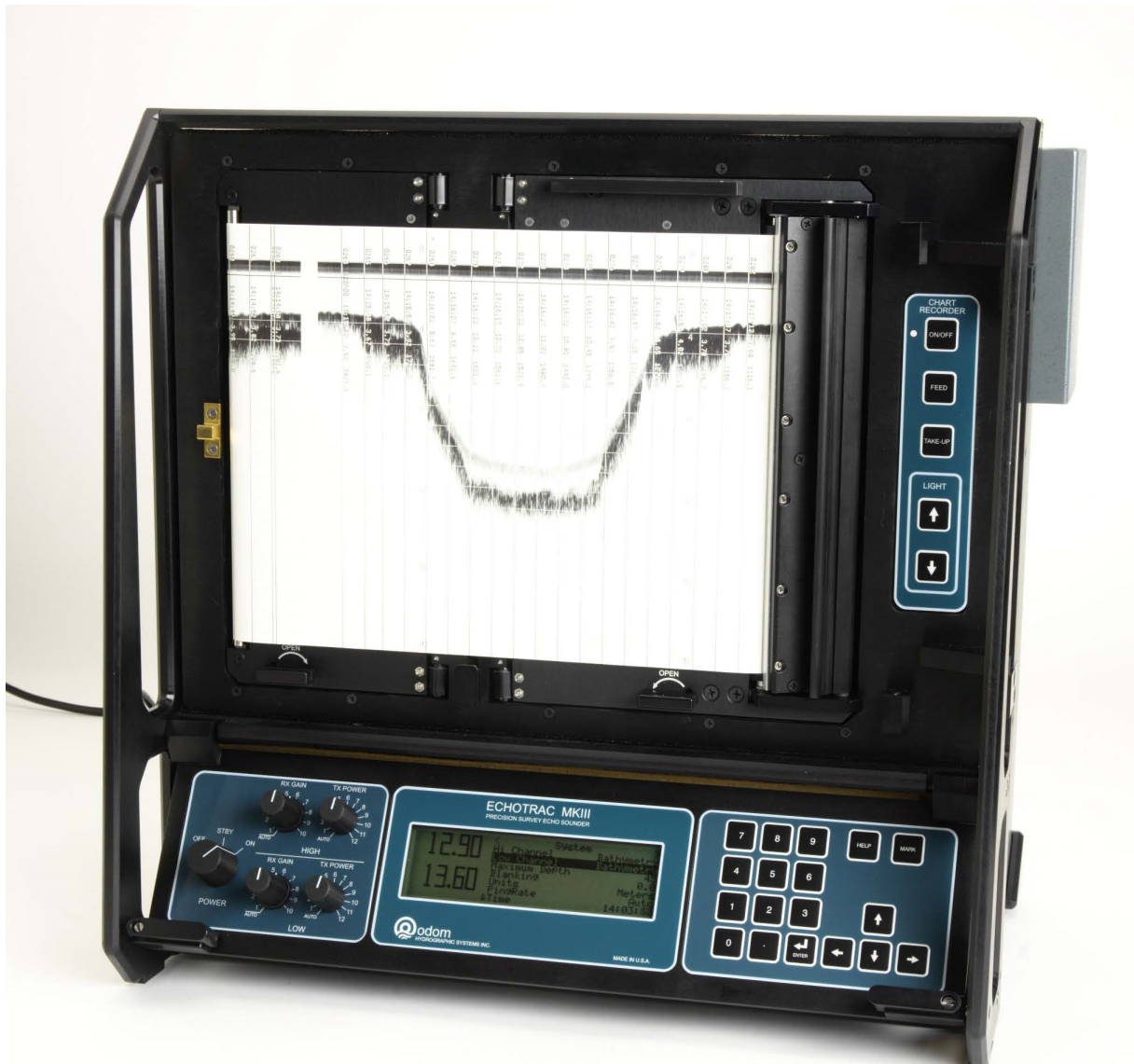
A dual frequency hydrographic grade echo sounder from Odom.
