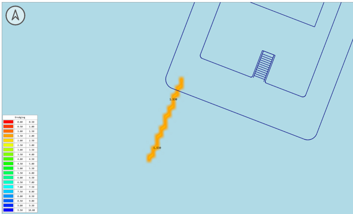
Example of recorded echo sounder data.
