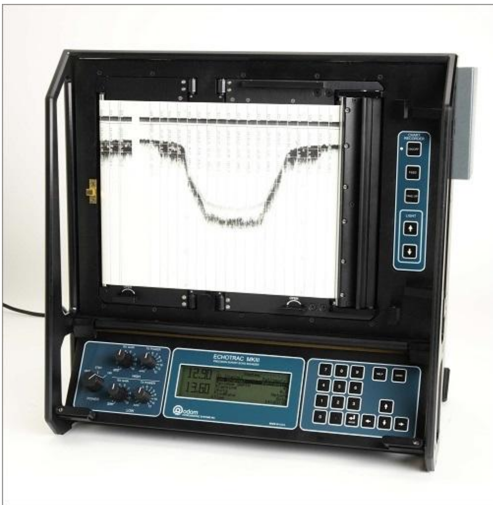
An echosounder capable of writing annotation marks to thermal paper (Odom EchoTrack).
